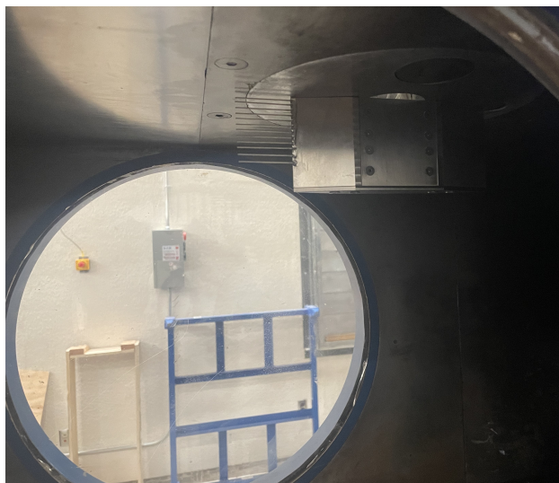
Figure 2.9: Boundary layer rake installed in APWT.
